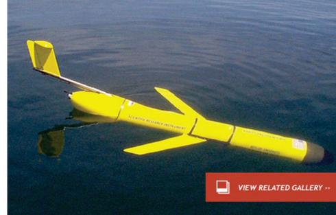
Aquatic drones, known as gliders, will soon surf the waves and dive into the deep from Nova Scotia to Georgia. The gliders will collect data during the peak of the Atlantic hurricane season. By recording conditions in the middle of a storm the gliders will help oceanographers forecast storm intensity during future storm seasons.
